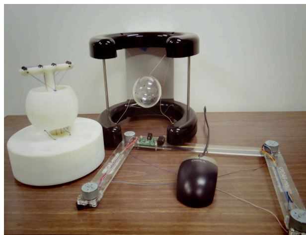
Figure 1: Desktop versions of the SPIDAR systems SPIDAR-I, SPIDAR-G and SPIDAR-mouse
