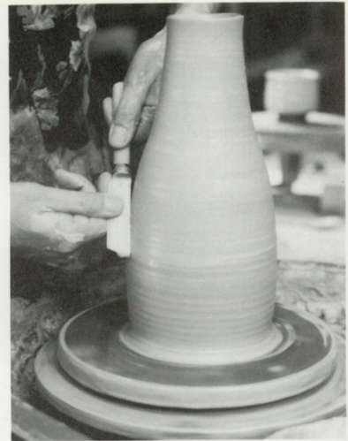
Ribbing and giving base its foot, which gives a better grip when dipping in slip or glaze
