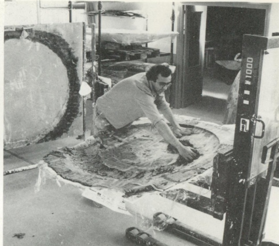
Casanovas working on dish supported on fork lift truck; other dishes are in the background. The fork lift truck will be used to carry the dish to the kiln and lower it in position
