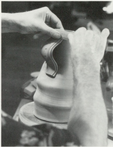
Top of handle secured by pressing with ruler
