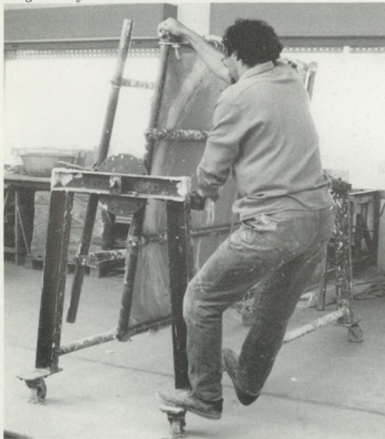
using double framework to turn 'dish' over
