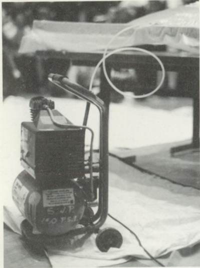
LEFT air compressor maintaining pressure in bladder: RIGHT Casanovas laying plaster soaked hessian strips over dome at Aberystwyth International Potters Camp
